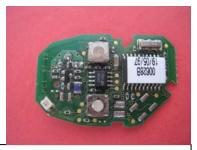
Open remote on the split line and separate electronic part from hard shell top part. Remove old rubber insert and any remnants of the old rubber key button from the shell. You can use small flat screw driver.
